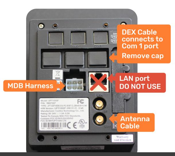
There are only 3 connections that need to be used on the Engage device.
