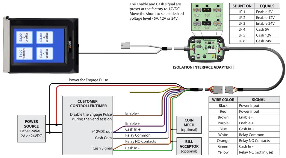
**ENGAGE PULSE POWER:** The Red and Black wires are used to power the Engage. Either a 24VAC, 2A or a 24VDC, 2A power supply is recommended.
